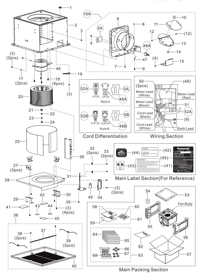
Remark: Please take attention to the parts which circled with broken line, We express the different style parts in using a letter marked behind a number, such as 5A means the item 5 belongs to style A.
