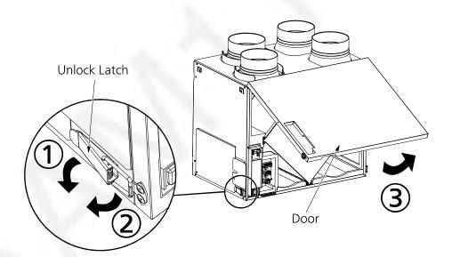
Clean the OA filter, RA filter and energy recovery core.
