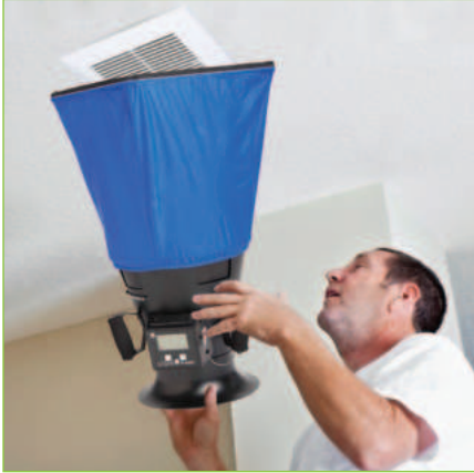
Balometer used to verify installed performance
