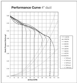
\*Industry research indicates static pressure in typical installations ranges from 0.20\* to 0.37
