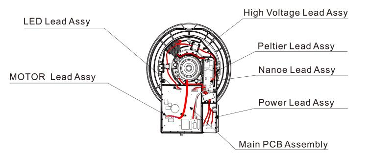
When replacing the Lead Wire or Main PCB, please be sure to hold the Main PCB in place before pulling out the lead wire. Otherwise the PCB may be deformed or damaged because it does not have screws.
