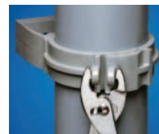
2-1/2" to 4" Press pipe into QuickLATCH, up to the first notch to lock it in place. Then squeeze tabs together for a super-secure hold.
